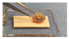
• The back plate is placed on the stem of the front plate.
