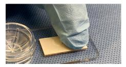
• The back plate is gently pushed down with a finger onto the stem.
