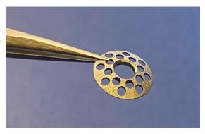
• The back plate (8.5 mm diameter) with a central hole, and 16 holes (1.2 mm each)
