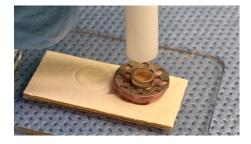
• The hollow end of the assembly tool is used to press the locking ring firmly down into the groove, usually with an audible snap. The assembly tool must be at 90 degrees from the front plate when pressing down.
