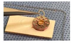
• The locking ring is placed on the stem of the front plate and properly aligned parallel to the front plate prior to final assembly.
